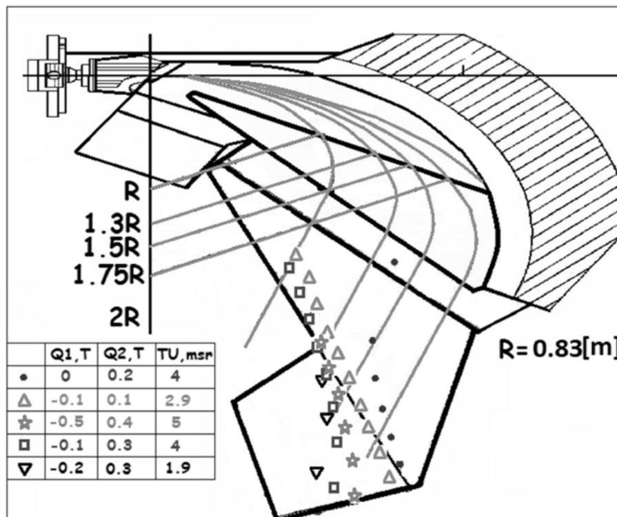
Figure 2. Graphic representation of the reconstructed focal planes of the MAVR analyzer in MAVRPC++ for the central particle with  $BP_0 = 0.91 \text{ Tm}$  with different fields of quadrupoles.
