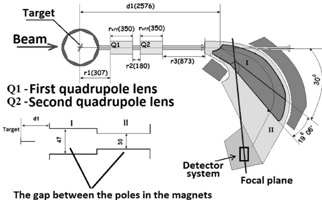
Figure 1. Conceptual scheme of the MAVR high-resolution spectrometer.
