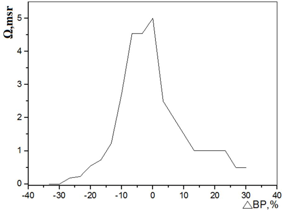
Figure 3. Dependence of the effective solid angle of the MAVR facility on the relative stiffness of the BP/BP0 particles for a  $60 \times 60$  mm detector system.
