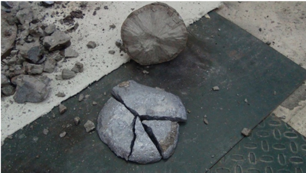
Figure 2. Homogeneous phase of silicon formed on top of the slag.
