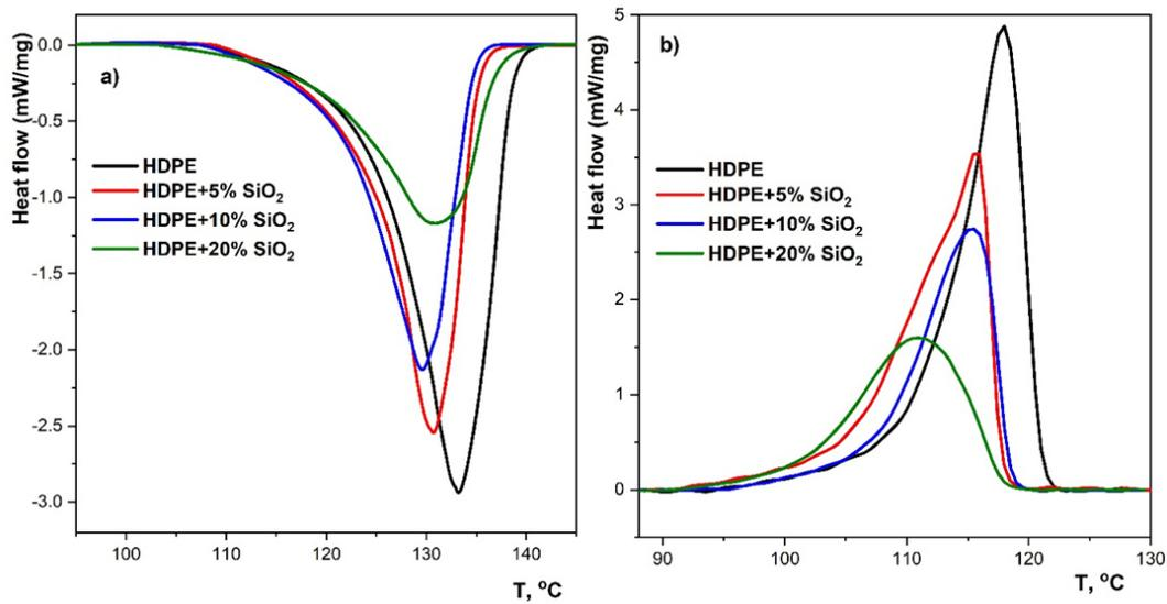
Figure 4. DSC thermograms for the pure HDPE and the HDPE+%SiO<sub>2</sub> nanocomposites: (a) 2<sup>nd</sup> heating and (b) 1<sup>st</sup> cooling cycles.
