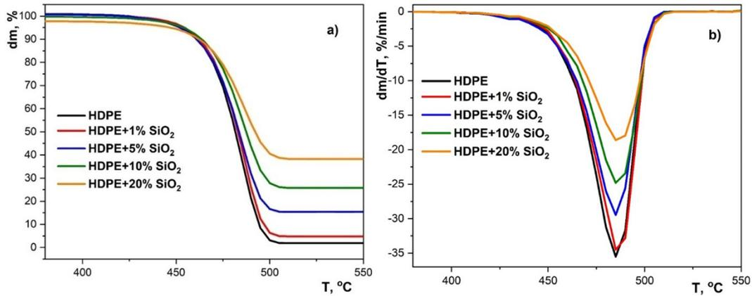
Figure 5. TGA curves (a) and its first derivative curves versus temperature (DTG) (b) of HDPE+%SiO<sub>2</sub> nanocomposite films.
