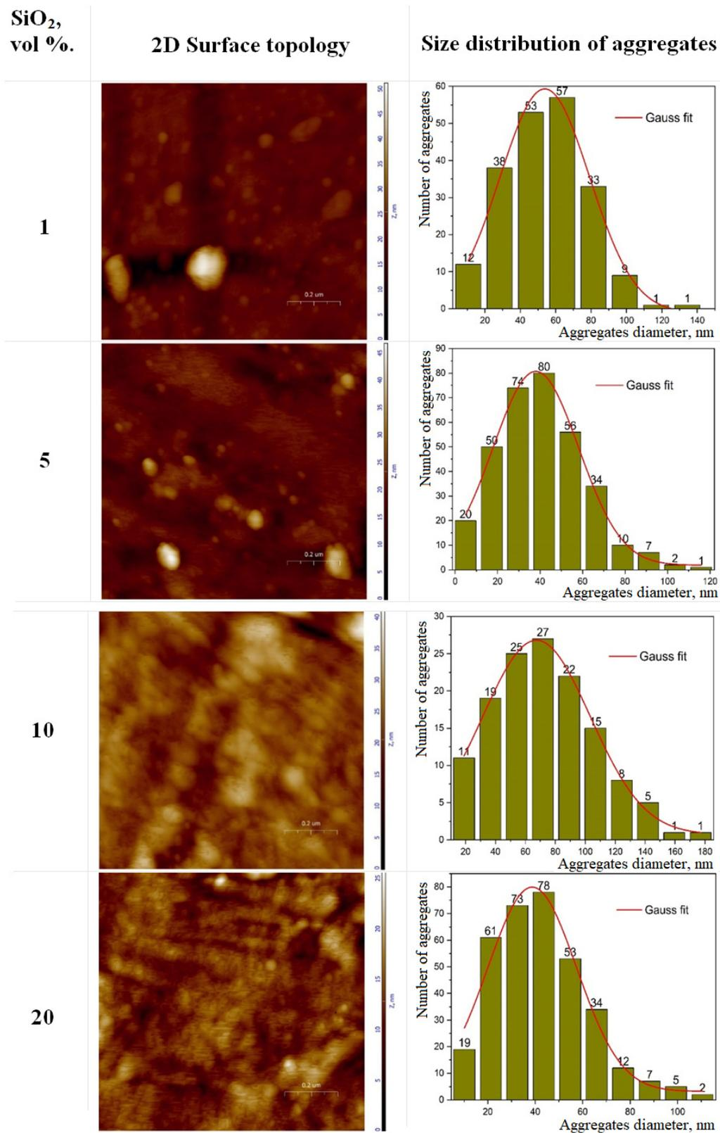
Figure 1. The surface topology images of HDPE/SiO<sub>2</sub> nanocomposites and size distribution of aggregates of SiO<sub>2</sub> nanoparticles.
