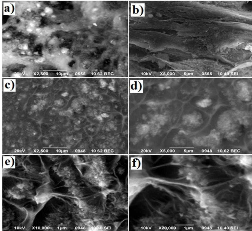
Figure 3. The fracture surface morphologies of HDPE+10%SiO<sub>2</sub> polymer nanocomposite films: (a) and (c) - × 2500; (b) and (d) - × 5000; (e) × 10000; (f) × 20000.
