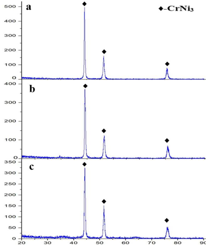
Figure 3. Diffractograms of the NiCr coatings received at filling 58% (a), 54% (b), 65% (c).
