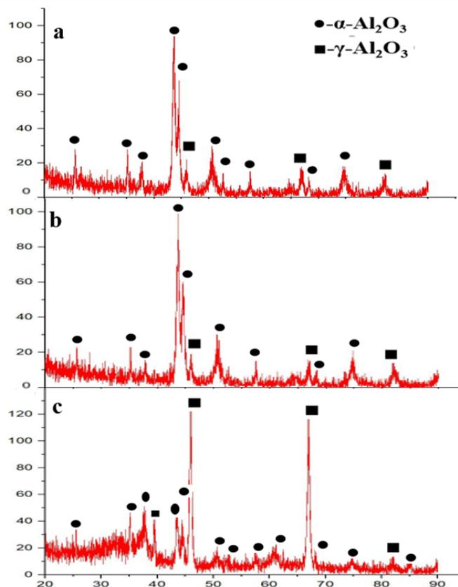
Figure 2. Diffractograms of  $\text{Al}_2\text{O}_3$  coatings obtained at barrel filling volume 63% (a), 54% (b), 45% (c).
