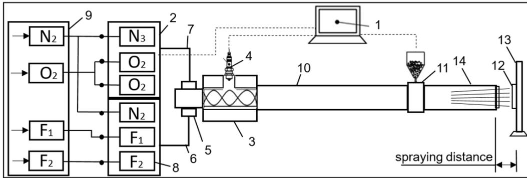
Figure 1. Schematic diagram of CCDS2000 detonation system: 1-control computer, 2-gas distributor, 3-mixing-ignition chamber, 4-spark plug, 5-barrel valve, 6-fuel line, 7-oxygen line, 8-gas valves, 9-gas supply unit, 10-breech block, 11-powder batcher, 12-workpiece, 13-manipulator, 14-muzzle of the barrel.
