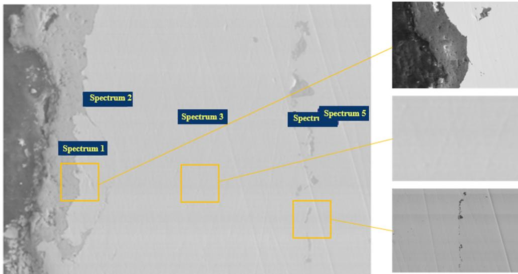
Figure 4. SEM cross-sectional image of multilayer coating on the bases of NiCr/NiCr-Al<sub>2</sub>O<sub>3</sub> / Al<sub>2</sub>O<sub>3</sub>.
