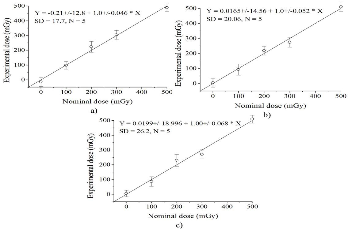
Figure 5. Dependence of Experimental dose from nominal dose for four repeated spectra measurements (a)- for measurement conditions after 17 o'clock without mobile phone; b)-for measurement conditions from 9 to 17 o'clock without mobile phone; c)-for measurements conditions with mobile phone).
