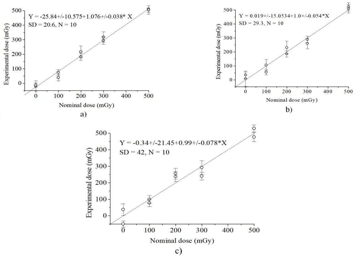
Figure 4. Dependence of Experimental dose from nominal dose for single spectrum measurement (a) - for measurement conditions after 17 o'clock without mobile phone; b)-for measurement conditions from 9 to 17 o'clock without mobile phone; c)-for measurements conditions with mobile phone).
