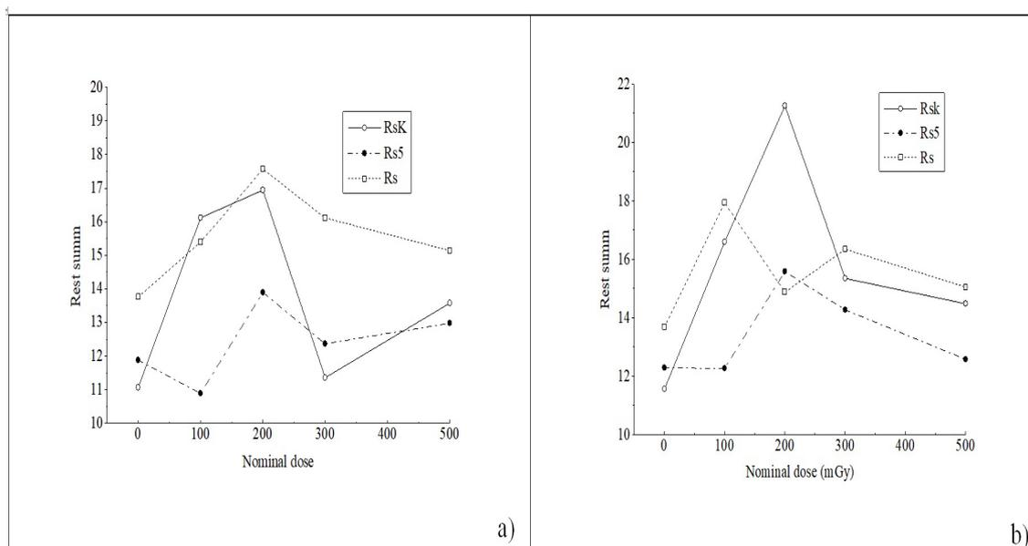
Figure 3. Dependence of rest sum from nominal dose?(a-for single spectra measurements; b-for average of four repeated spectra measurements; RsK-residual signal for measurements conditions with mobile phone; Rs5-residual signal for measurements conditions after 17 o'clock without mobile phone; Rs-residual signal for measurements conditions from 9 to 17 o'clock without mobile phone).
