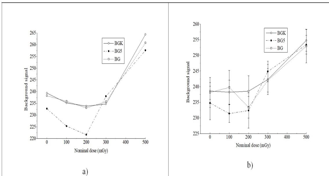
Figure 2. Dependence of background signal from nominal dose (a-for single spectra measurements; b-for average of four repeated spectra measurements; BGK-background signal for measurements conditions with mobile phone; BG5-background signal for measurements conditions after 17 o'clock without mobile phone; BG-background signal for measurements conditions from 9 to 17 o'clock without mobile phone).
