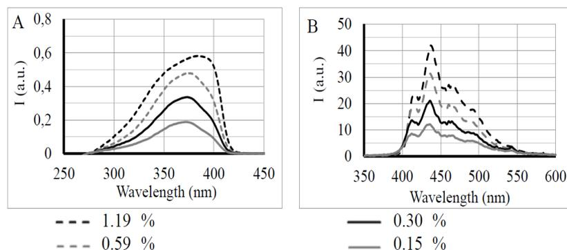
Figure 2. Spectra of absorption (A) and fluorescence (B) of PVA samples containing St420.
