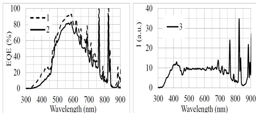
Figure 5. Spectrum of emission of solar light simulator (1), calculated based on EQE spectrum of effective absorption of SC (2) and difference of spectra 1 and 2 (3).
