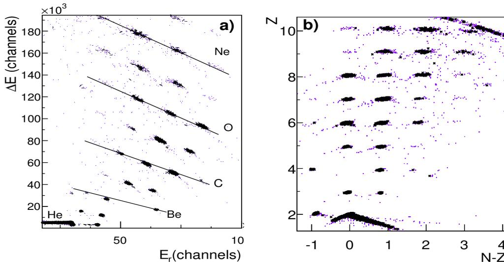
Figure 1. a) Particle identification plot for the products of the ( $^{48}\text{Ca}+\text{Ta}$ ) reaction from  $^4\text{He}$  upto Ne-isotopes.  $\Delta E$  is the energy loss and  $E_r$  is the residual energy. b) Identification matrix (product yield versus atomic number  $Z$  and neutron excess  $N-Z$  values) obtained by so-called ( $\Delta E \times E$ ) method.
