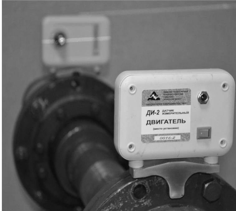
Figure 3. Wireless alignment system "PC-Lazer-V".
