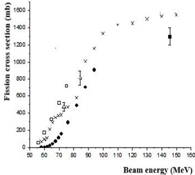
Figure 2. Fission cross section : □ - data [2]-reaction ( $^{11}\text{B} + ^{209}\text{Bi}$ ), ● - data [13]-reaction ( $^{12}\text{C} + ^{208}\text{Pb}$ ), △ - data [16]-reaction ( $^{12}\text{C} + ^{208}\text{Pb}$ ), ■ - present work, × - PACE-4 code calculation - reaction ( $^{11}\text{B} + ^{209}\text{Bi}$ ).
